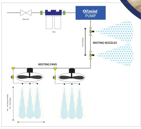
The high-pressure water is forced through a stainless steel mist nozzle that breaks the water into millions of tiny droplets that 'flash evaporate' and absorb the heat in the air without wetting any floors or surfaces.
