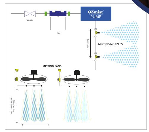
The high-pressure water is forced through stainless steel mist nozzles creating millions of tiny droplets that absorb the latent heat in the air. Leaving the curtains open slightly ensures that humidity levels do not increase beyond acceptable levels. The mist totally evaporates before wetting pigs, floors or feed equipment.
