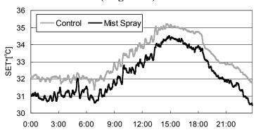
c) Spraying to the outdoor unit of room air conditioner. A representative result for spraying to the outdoor unit of room air conditioner is shown in Figure 8, which shows the effect on reduction of electricity consumption for air-cooling on September 22. On this day, energy consumption in the test apartment was 34.3% lower than the control room. The average reduction in energy consumption during the test period was 36%.
