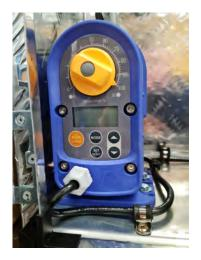
Connection of the odour dose to the misting pump module
