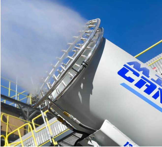
Atomised 'mist' released at 1000psi pressure
